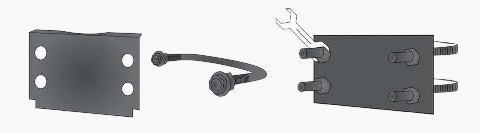
Insert the rod in the slot created between the weather station and the U Clamp
