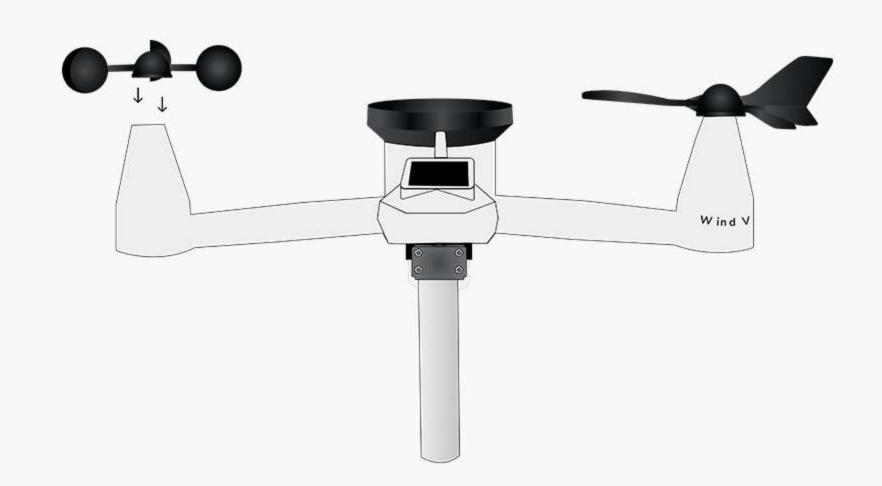
Close the top of the anemometer with the rubber plug provided in the kit.
