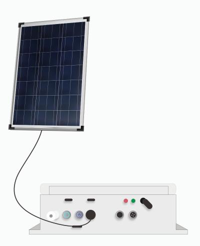
Position the solar panel at a 30-degree angle for perfect sunlight exposure to power the device.
